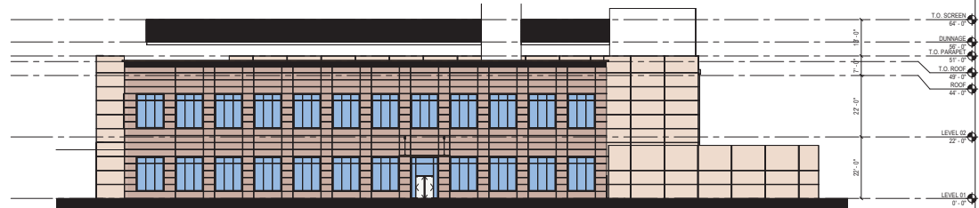
01 WEST ELEVATION (typical street facing) SCALE: 1/16" = 1'-0"
